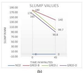
Fig. 1 Slump value of concrete (a) OPC and (b) PPC with different water reducing admixture
