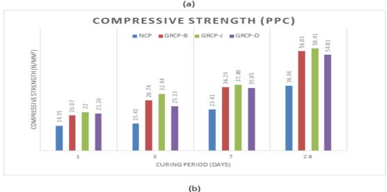
Fig. 2 Comparisons of strength 1, 3, 7 and 28 days of concrete with admixtures and normal concrete.
